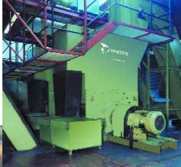
Example of a turnings crusher installation with feeding and discharge conveyors in the metalworking industry
