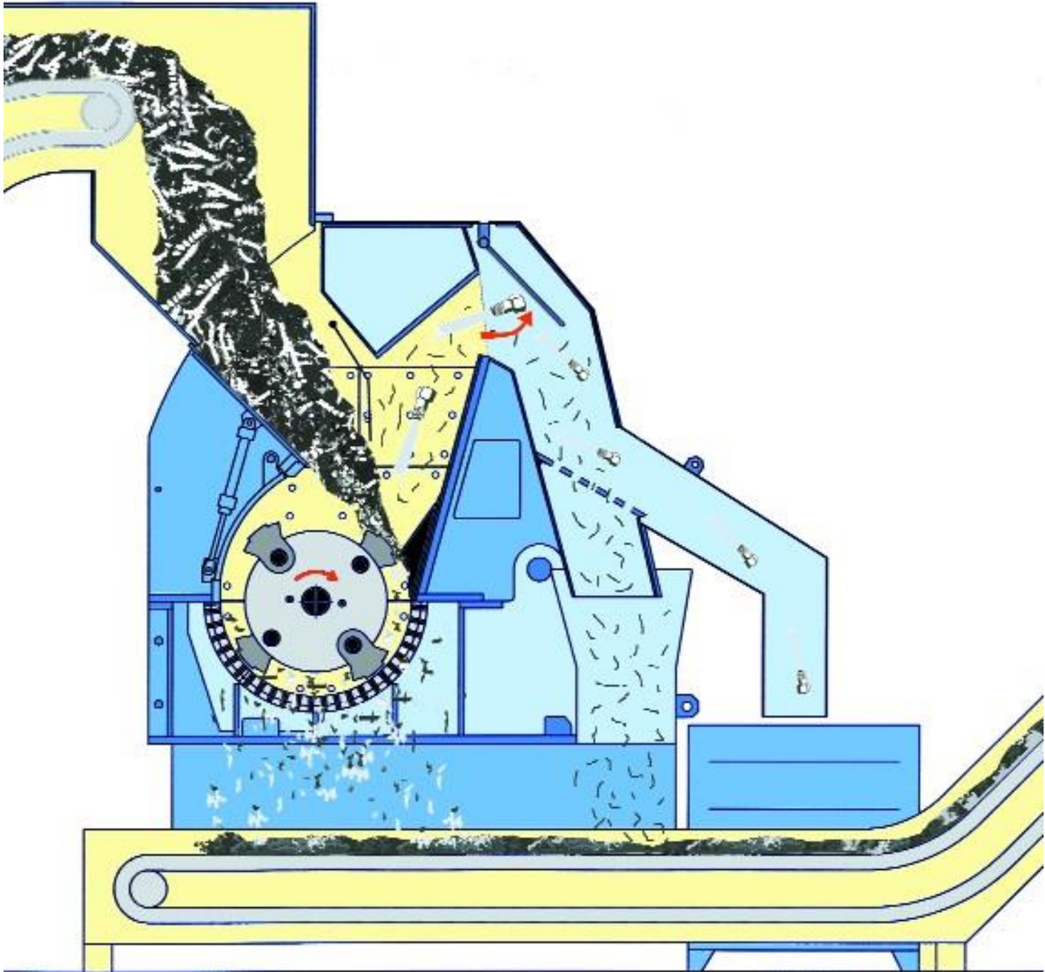
Lindemann ZB116 with additional grid in the coarse-pieces channel for screening out fine turnings
